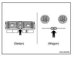
The hazard warning flasher button is located on the center of the instrument panel.
